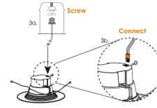
3b. Connect the orange connector of the Edison socket adapter
